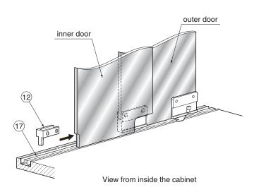
Insert support fixing ② in the bottom guide rail ⑦. Slide support fixing ② and affix to the inner door.
