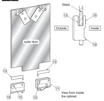
Glass lock ① and right guide ⑨ installation Both the glass lock (1) and right guide (9) should be placed so that the screws (5) are facing the inside of the cabinet. Ensure that gaskets (13) are placed between the outside face of the glass and the hardware as shown above.
