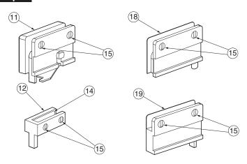
Ensure that parts 11/12/18 and 19 each include 2 screws (5). Similarly check that gasket (4) is affixed to glass support fixing 12.
