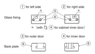
Make sure that the gaskets ⑥ and boss covers ⑤ are on glass fixing ① and ② as shown in top drawing. Glass fixing metal fittings ① and ② are reversed parts for left and right sides. Check that one of each ① and ② and the corresponding back plates ③ are provided.
