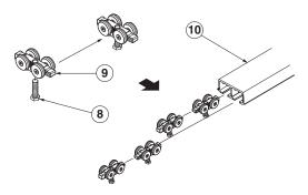
Assemble upper roller (9) and roller axial bolts (8) and insert them in upper rail (10) as shown above.
