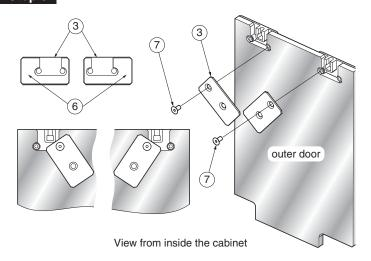
Do not remove protective paper backing from gasket attached to back plate 3. With a hexagon (allen) key, nominal size 4, temporarily fix back plates. Fix only inner screws. Repeat all instructions to this point for inner door of the cabinet.
