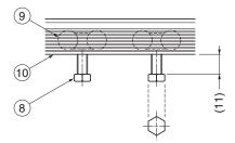
Adjust height of roller bolts ® and orient the head as shown on the drawing on the left.
