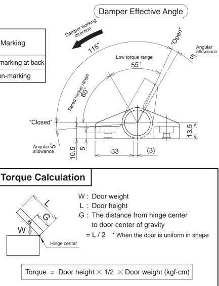
Even when the hinges are manually turned in the rated torque range (0 to about 60 degrees), it automatically returns to about 60 degrees when it is released. Fit the door at an angle at which the hinges do not automatically return (low torque range-about 60 to 115 degrees) even when they are released (see (Damper Effective Angle)).
