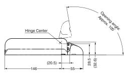
Fixing screws are not included. Please prepare for screws with suitable length.
