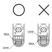
Confirm that upper roller is not dislocated from casing, for both door sides.
