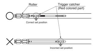
If the position is wrong, pull back the trigger catcher to the correct position using 6mm diameter round hard bar.
