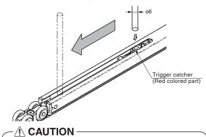
It may cause a failure of self-closing without confirmation of installation.
