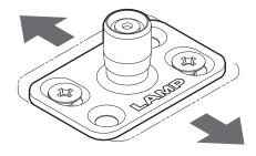
Tighten all 4 screws after the adjustment.
