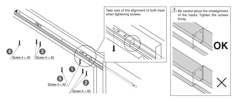
After fixing the track, move rollers and check if there's any misalignment or gap between the tracks.
