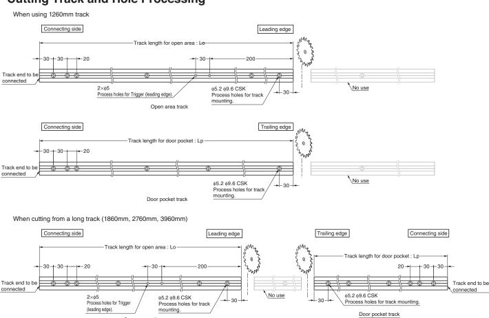
When cutting, use reinforcer for the track to prevent deformation at cut section.
