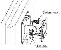
Caution Lock lever may pop out if you try to move the monitor when it is locked. Do not move the monitor when it is locked.
