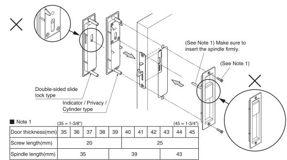
Change the screws and spindle according to the door thickness.
