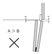
If "A" is bigger than "B", the closing action would not be smootht. Re-adjust the gaps as below.
