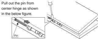
7 Fixing the mounting plates for Pivot side
