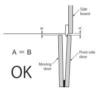
Adjust the fore-and-aft position of the concealed hinges so that the both A and B gaps are the same.
