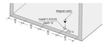
For metal cabinet, drill a hole at a position of a quarter of the opening width, as shown in the right figure.
