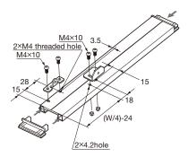
Make threaded holes to fix Spring plate to End-slat.
