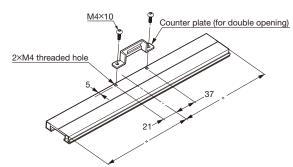
Pay attention to the direction of End-slat and the positional relation between End-slat and Counter Plate.
