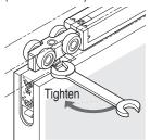
When vertical frame is not used, install door stopper, without fail.
