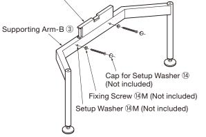
**7** Assembling of Interlocking Arm (1) and Fixing of Supporting Arm-A (2)
