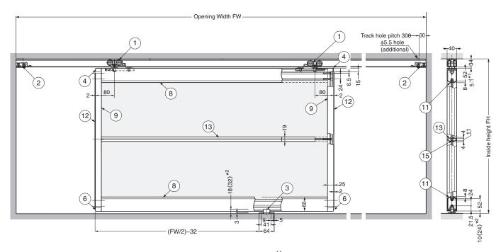
$<sup>^{\</sup>star 1}$  Height adjustable range : -4 mm to +1 mm  $^{\star 2}$  Dimension ( ) : when floor guide : when floor guide L16 (optional) is used.
