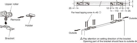
Opening part of the bracket should face to outside direction.
