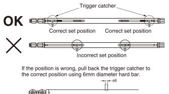
1 If the closer is installed without conformation, it will cause the trouble such as no-sliding of door.
