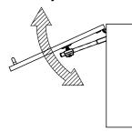
·Attach the Slider with the fixing bolt M4x5
