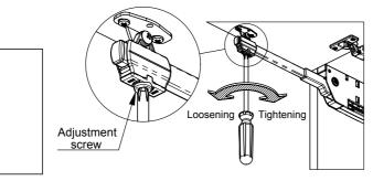
· If you feel that the door is too light (self lift-up) or too heavy (self-closing), it is possible to limit the action of the spring by tightening the adjustment screw.
