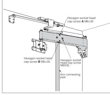
Tighten the Hexagon socket head cap screws on Lower arm. Adjustment would not be achieved if the screws on Lower arm were loose.
