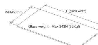
For glass thickness 8mm, L=1124mm would be the maximum, and thickness 10mm, L=1424mm would be the maximum.
