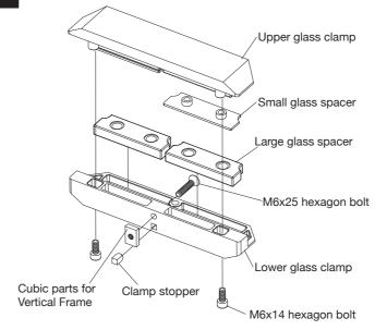
Please screw off the glass clamp by loosening the M6x14 hexagon bolt.
