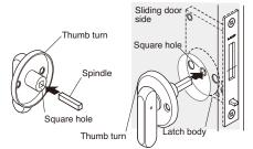
3 Mounting Indicator / Emergency Release Insert Spindle into Indicator or Emergency Release
