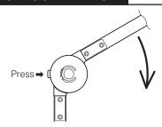
Press and hold release button just before the desired angle, then release the button and turn the stay until it is locked.
