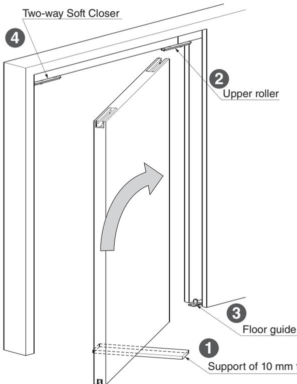
Insert the upper roller into the hanging bracket in the door. Position upper roller hanger bolt to 80mm from door edge (41 mm to fix plate edge). Tighten fix bolt with Spanner ⑪.
