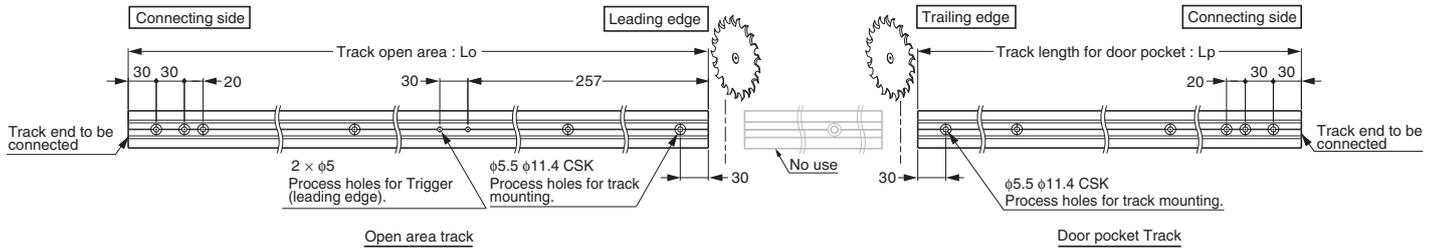
**!** When cutting, use reinforcer for the track to prevent deformation at cut section.
