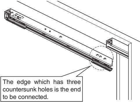
Overlap the two countersunk holes on the Pocket trigger and the two holes on the Upper track nearby the open area.
