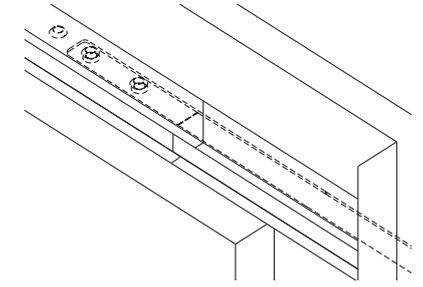
When sliding Pocket trigger, use a screwdriver.
