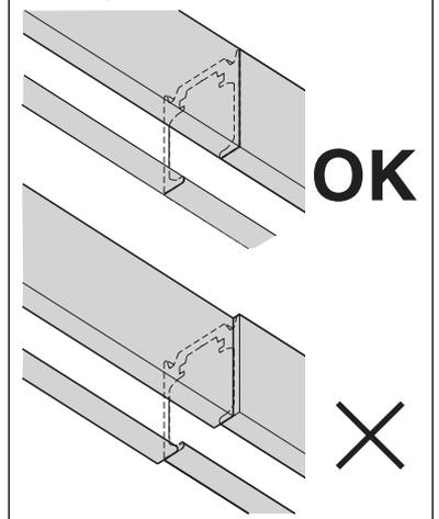
① After fixing the track, move rollers and check if there's any misalignment or gap between the tracks.
