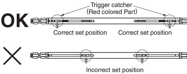
If the position is wrong, pull back the trigger catcher to the correct position using 6mm diameter hard bar.
