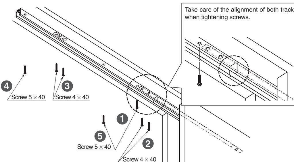
⚠ Be careful about the misalignment of the tracks. Tighten the screws firmly.
