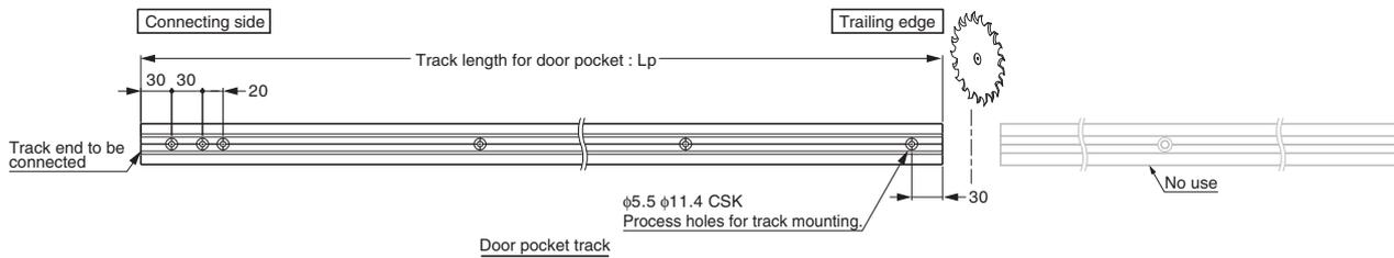
When cutting from a long rail (2160 mm, 2760 mm, 3960 mm)
