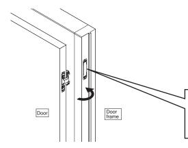
While holding the door, insert Hinge main body into the Base frame on Doorframe. Keep holding the door and fix the hinge with the fixing screws at once.
