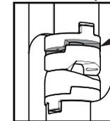
Check the hinge assembly before hanging the door. If there is a gap in the bush assembly, please turn the bush 180° and ensure that there is no more gap.
