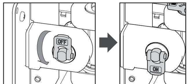
Above drawings show tilt lock. The way of swivel lock is the same.
