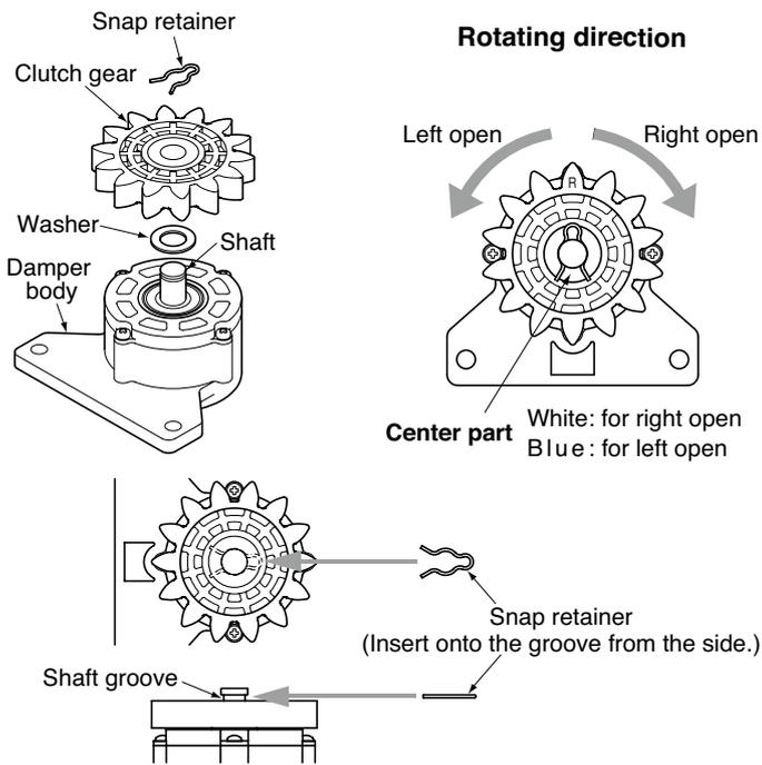
The braking device becomes non-handed by changing the direction of the clutch gear.
