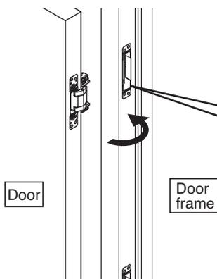
While holding the door, insert Hinge main body into the Base frame on Doorframe. Keep holding the door and fix the hinge with the fixing screws at once.
