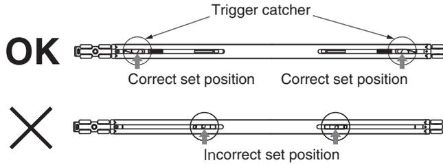
If the position is wrong, pull back the trigger catcher to the correct position using 6mm diameter hard bar.
