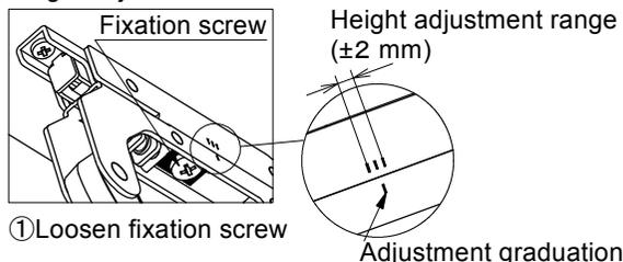
① Loosen fixation screw
