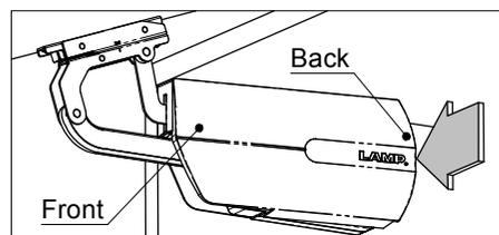
Clip the front and then the back of the cover. Make sure that the cover is securely attached. To remove, pull the back of the cover first.
