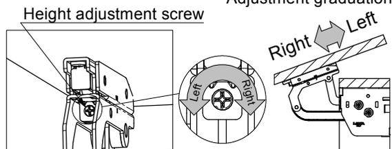
② Adjust height by turning the height adjustment screw as shown above. A graduation is visibly on the side of the mounting plate to show height adjustment.
