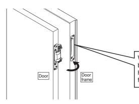
While holding the door, insert Hinge main body into the Base frame on Doorframe Keep holding the door and fix the hinge with the fixing screws at once.
