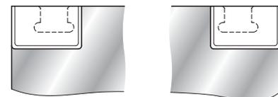
Remove protective paper backing from gasket ⑥ and fix the gasket to the glass as shown in left drawing.
