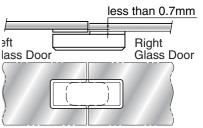
For smooth operation, we recommend to make sure of the doors parallelism. Moreover both doors depth alignment should be maintained within 0.7mm as shown above.
