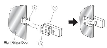
Insert the gasket (4) in the lock body (1) so that it will be located on the outer side of the cabinet. Then fit the lock body on the glass door and fasten fixing screws 3.
