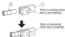
Insert key 5 in the slot of the lock body 1 as shown above in order to unlock. Simply remove the key 5 in order to lock. We recommend that you test the good operation of the rotor before proceeding to the final adjustments.
