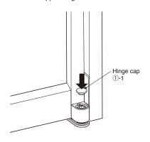
5-6. Attach the hinge cap ①-1 at last.
