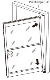
5-2. Insert the pin of the lower hinge ①-2 into the hole of the lower bracket. Guide the pin to the hole of the upper bracket, while pushing the pin of the upper hinge with your finger. Then, release your finger from the pin, and push the pin into the upper bracket. After setting it, ensure that the door cannot be removed even if it is pulled.
