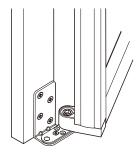
5-4. Securely tighten the lock ring in the upper and lower hinges ②.
