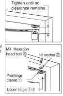
5-3. Tighten (up) the vertical adjustment screw of the lower hinge ①-2 until no clearance is left between the upper hinge ①-2 and the upper pivot hinge bracket ②. After the adjustment is complete, attach the locking flat washer ② and the hexagon head bolt ② to the upper hinge ①-2.
