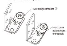
5-5. For horizontal adjustment, loosen the horizontal adjustment fixing bolt located at the upper and lower pivot hinge brackets ②, select one among the three holes, and re-tighten the bolt for fixing. Horizontal adjustment by 2 mm from the center is possible. (Tool: Nominal 3 Allen key wrench)
