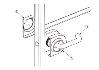
6-4. Install the strike <sup>®</sup> by gauging. Refer to the drawings shown below.
