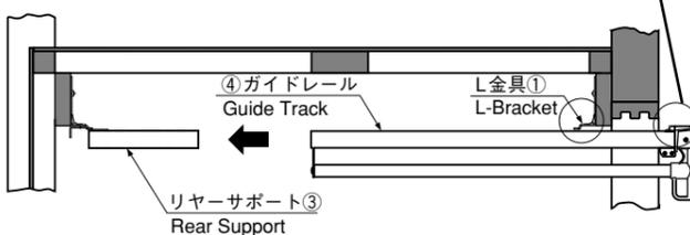
図(Fig.)5 MOUNTING OF GUIDE TRACK ⑤
