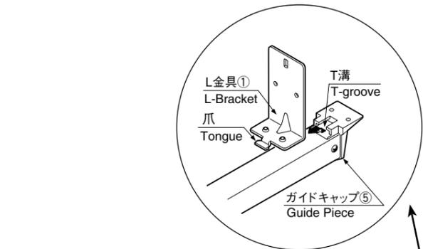
図(Fig.)4 MOUNTING OF GUIDE TRACK ④
