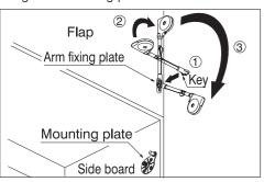
Turn the main body 90 degrees (2)  $\rightarrow$  3) and insert the pin of the mounting plate in the hole of the main body.
